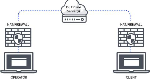
Diagram of Standard Connection using an ISL Conference Proxy (ICP) server to manage both the Control Channel and the Remote Desktop Data Stream.
